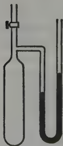
Fig. 15-4. Dissociation of calcium(II) carbonate
