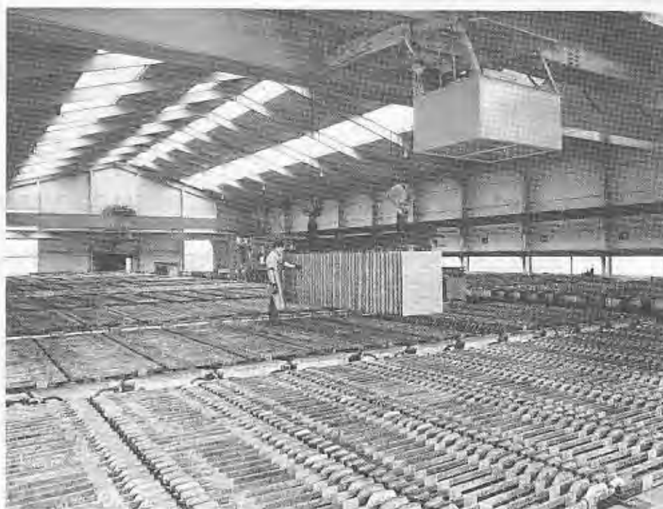
FIGURE 12.4 Purification of Copper by Electrolysis
