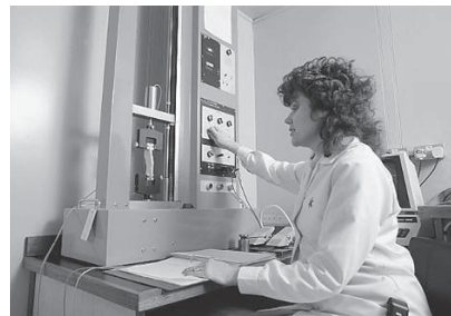
Fig. 7.12 A tensometer in use
