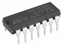
Fig. 16.4 A quad 2-input NAND chip. (Reproduced with the permission of Maplin Electronics.)
