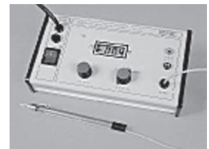
Fig. 18.22 A calibrated Hall probe
