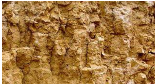
(iv) Columnar soil structure
