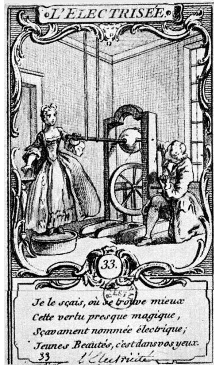
Typical friction machine using a glass globe, common in the 18th century
