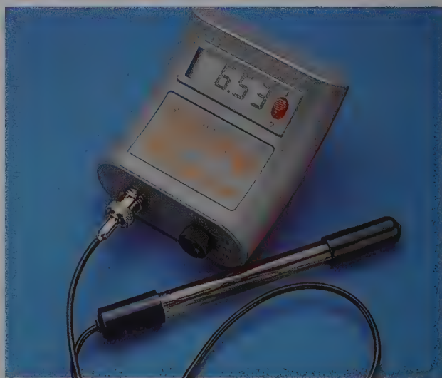
Figure 6.5 Measuring pH electrometrically
