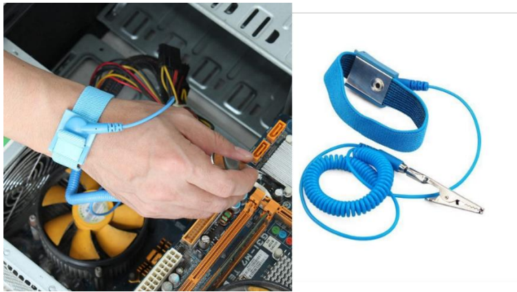
Figure 40: A technician wearing an anti-static wristband while installing RAM inside a desktop system
