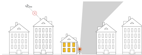
Incorrect placement with blockage – bad or no ADS-B signal reception
