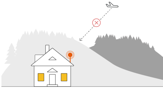
Bad position - hills blocking antenna
